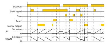
Timing starts when the start signal goes ON.
