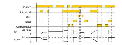
Start signal enables timing (timing is stopped when the start signal is OFF or when the power is OFF)
